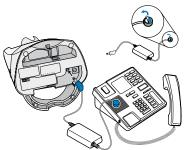
Connect the RD-1 POD cable to the headset base as shown; peel the adhesive off the back of the RD-1 microphone and attach to the telephone speaker.
