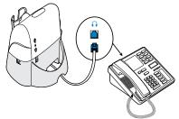
Connect the audio cable included with and pre-attached to the headset base to the headset port on telephone.
