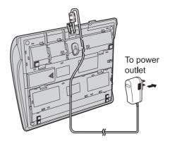
3 Dress the telephone line cord as shown. Tuck the telephone line cord inside the wall mounting adaptor, then push it in the direction of the arrows (① and ②).
