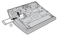
2 Match the polarity and snap the battery to the battery snap as shown.
